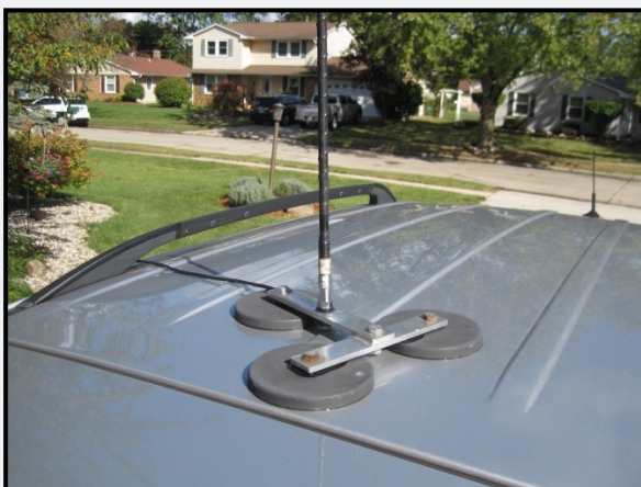
Typical 3 magnet antenna mount.
