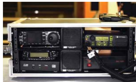
N9MTF Go Box With DMR Installed
