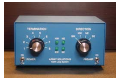
Figure 2. Control Box for Two K9AY Loops
